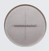
Eyepiece scale micrometer.
